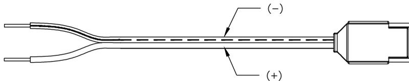
**Cable Polarity Detail**
