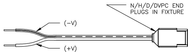
**Cable Polarity Detail**
