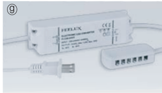
g LED Driver with 6way distributor, with power cord (70 55/64'') Part No FLC15-24V/XL FLC30-24V/XL FLC75-24V/XL Capacity 15W 24V 30W 24V 75W 24V
