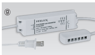
⑨ LED Driver with 6way distributor, with power feed(70 55/64") Part No FLC15-24V/XL FLC30-24V/XL FLC75-24V/XL Capacity 15W 24V 30W 24V 75W 24V
