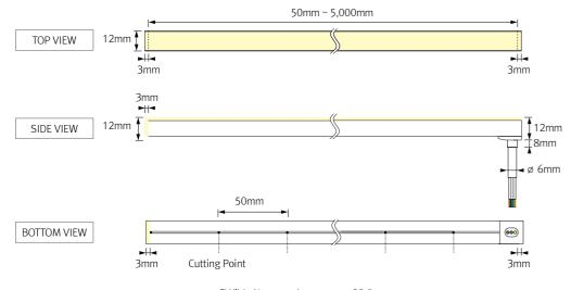
FLXible Neon can be cut every 38.5mm. Please follow the cutting point mark to cut precisely as needed.
