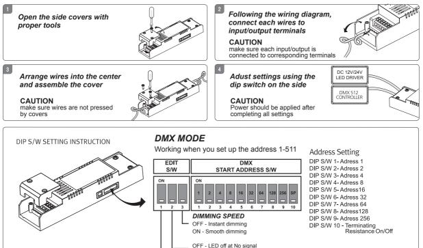
Working Test mode when you set up the address 0 When EDIT 1 time, S/W 2 times on/off in 5 seconds, Indicater LED is ON/OFF
