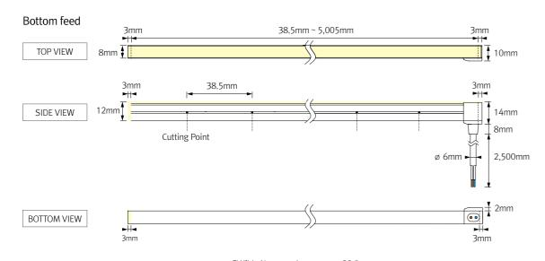
FLXible Neon can be cut every 38,5mm. Please follow the cutting point mark to cut precisely as needed.
